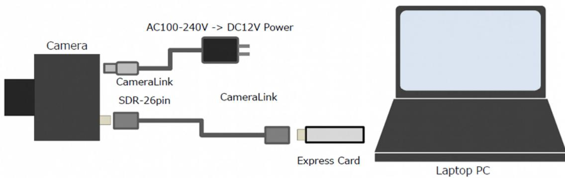
\*There is an unique port of CameraLink channel used since this camera operates with CameraLink - Base Configuration.
