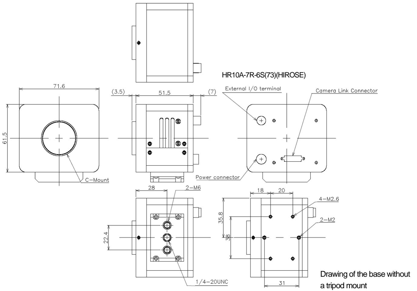
6.1.3. Schematic Diagram of the Sensor
