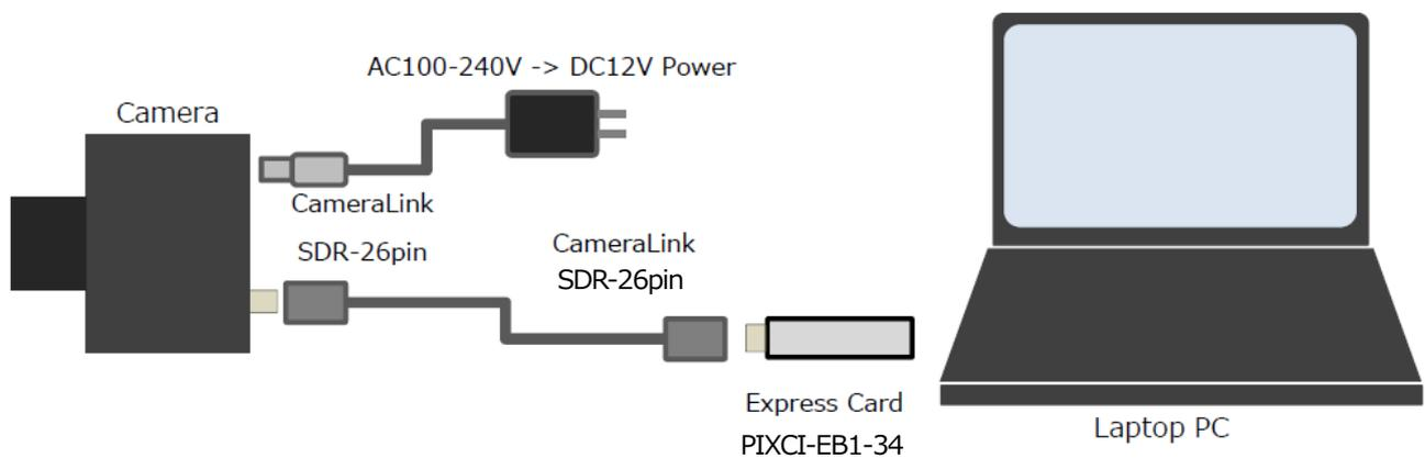
\*There is a unique port of CameraLink channel used since this camera operates with CameraLink - Base Configuration.
