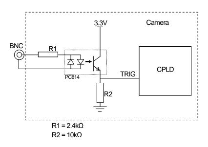
**Trigger Input Circuit**
