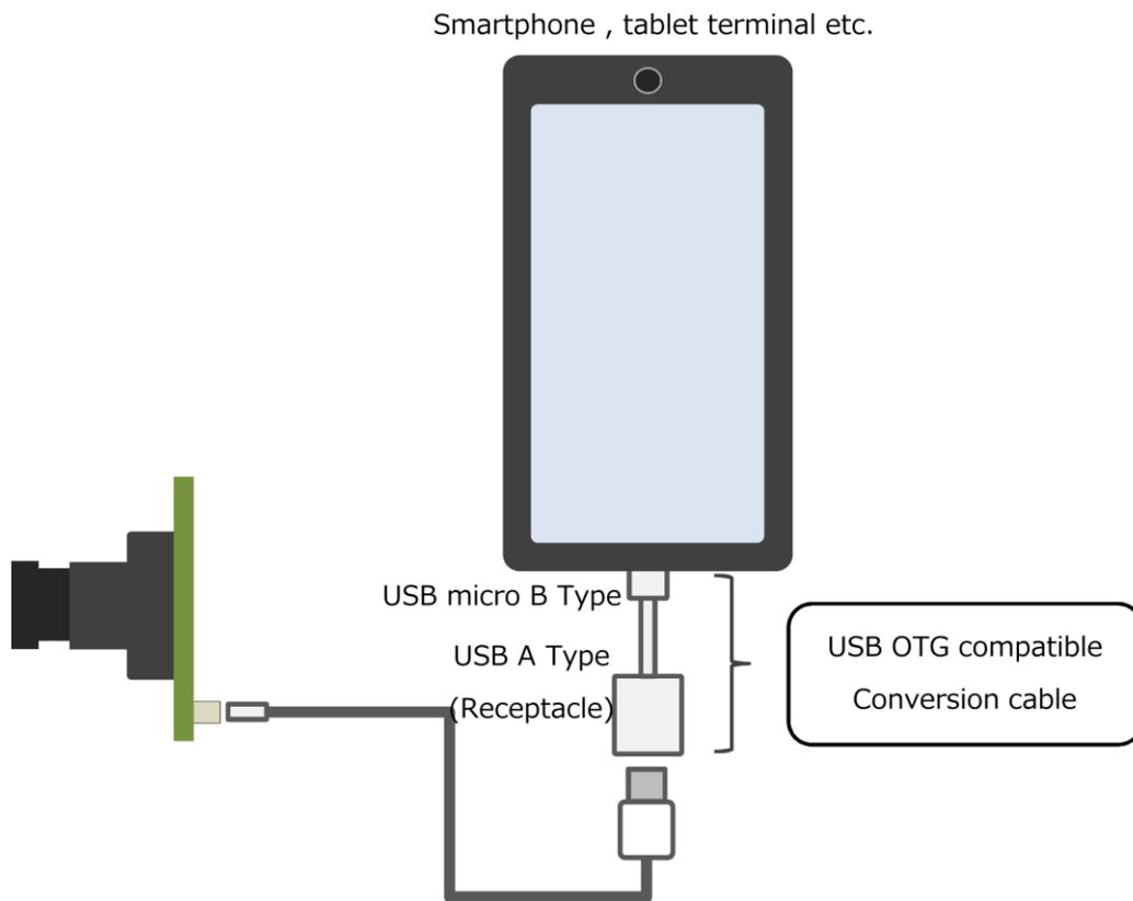
When connecting multiple cameras, connect a USB hub with a USB OTG compatible cable and a USB A-B cable, then connect the USB hub and camera with the included USB 2.0 cable.
