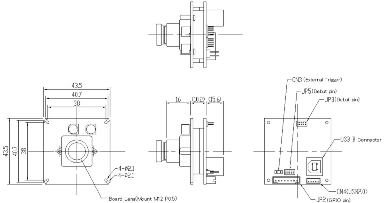
\*Depending on different models, size and position of components in front of sensor board (condenser...) might vary.
